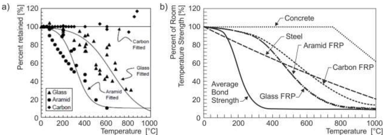
Fig. 3. Approximate variation in tensile strength and bond strength with temperature increase; a) Bare fiber strength [10]; b) FRP, concrete and reinforcing steel [11]
