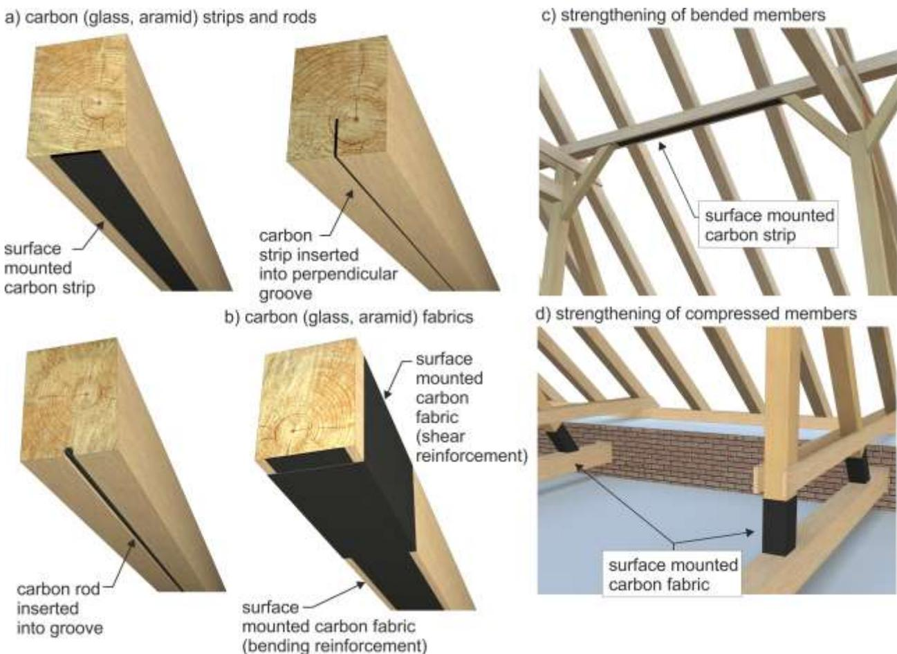
Fig. 1 Examples of strengthening of timber structures using externally bonded FRP materials (EBR)
