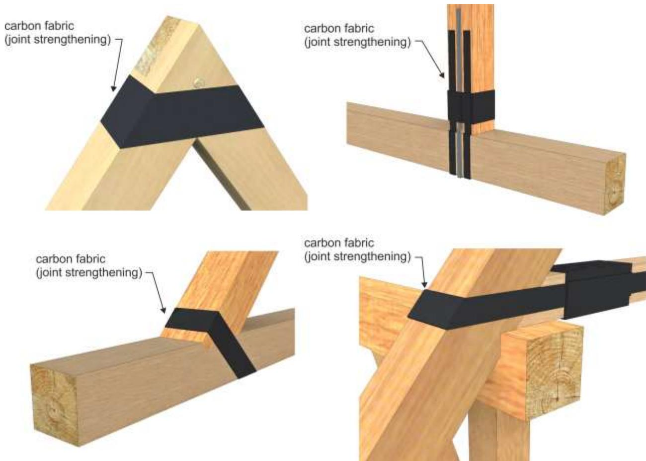
Fig. 2 Examples of possible joint stabilization and strengthening using externally bonded FRP materials (EBR)
