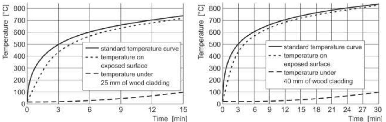
Fig. 5 Temperatures at the FRP reinforcement in case of fire protection system using wood cladding 25 mm (left) and 40 mm (right) thick
