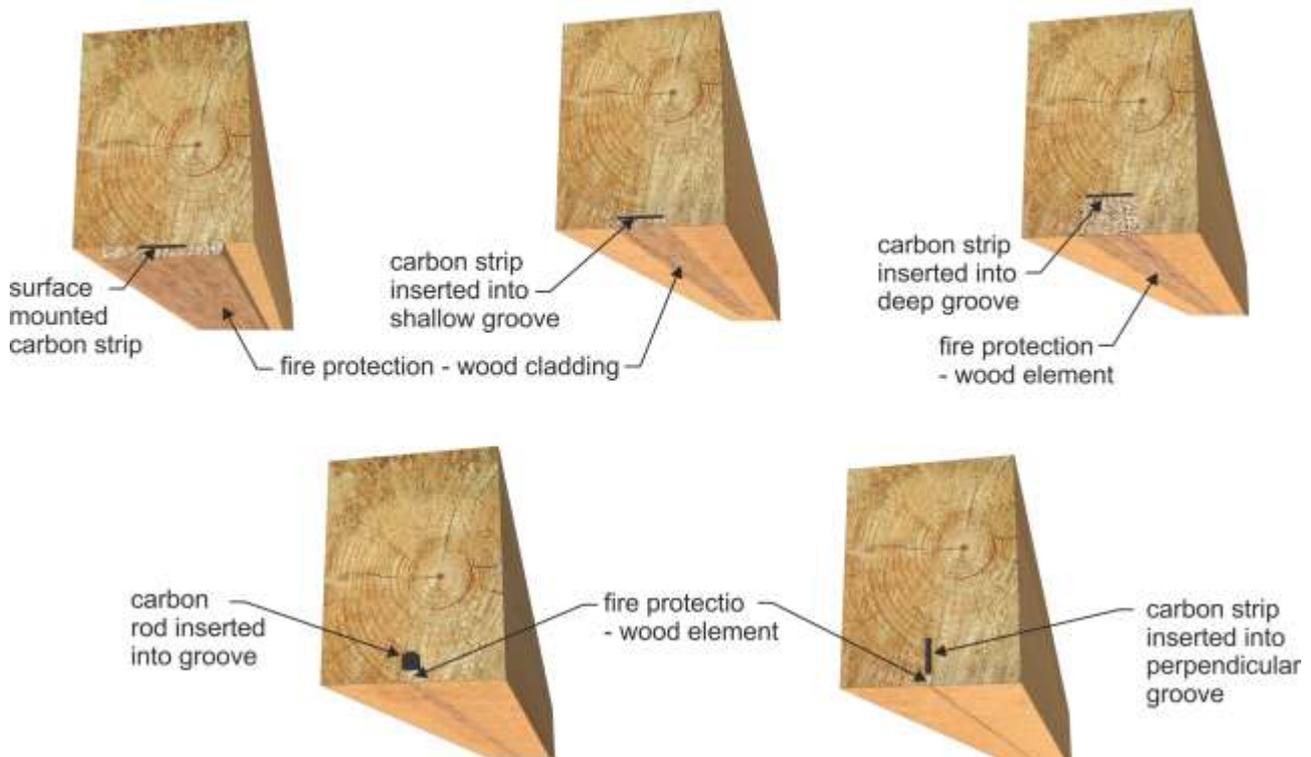
Fig. 4 Fire protection of strengthening FRP elements
