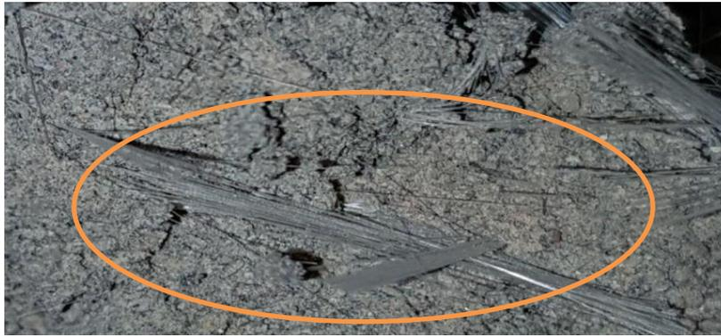
Fig. 5 - The view of how FN-fibers and soil interlocked, application of FN-fibers for preventing crack in loading moment
