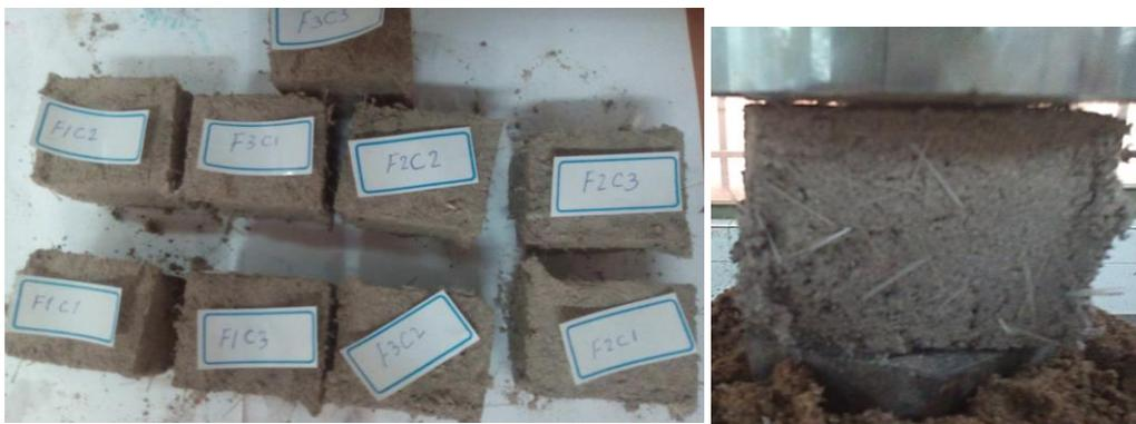
Fig 4- Stabilized sand samples with cement and reinforced with FN-fibers (right). Close view of reinforced and stabilized samples (left)
