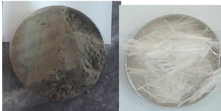
Fig. 3 - A view of the Portland cement type II (left), and FN-fiber (right)
