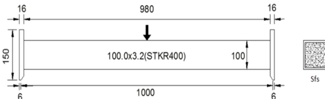
Fig. 1 – Specimen's Illustration (unit: mm)
