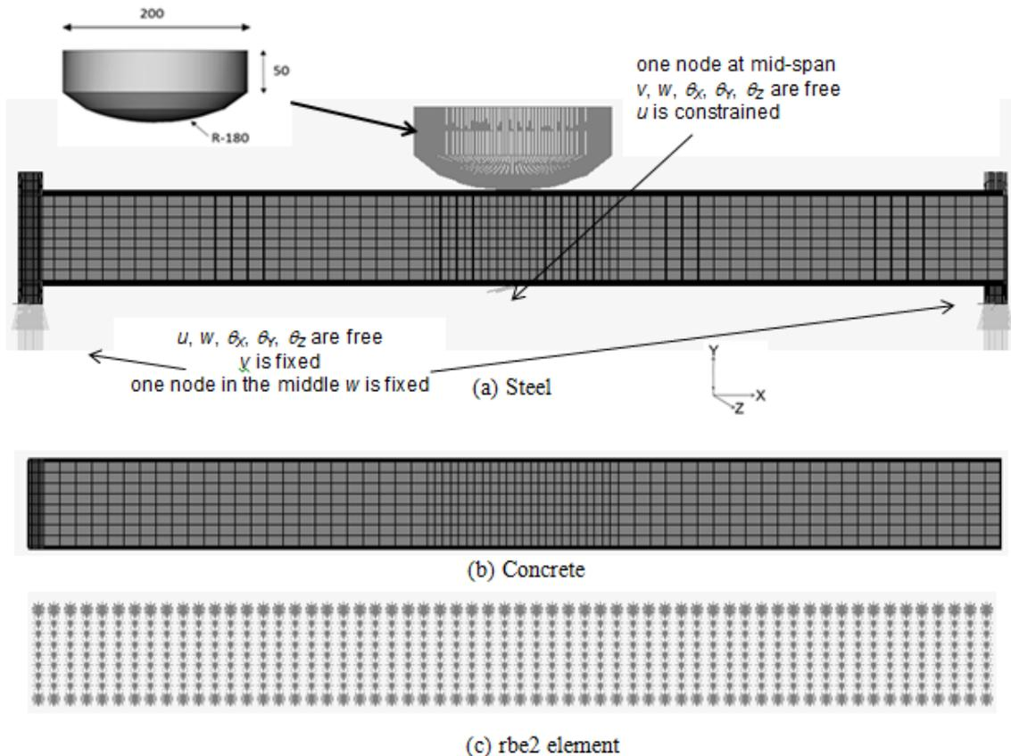
Fig. 7 – Boundary Conditions and Mesh Segmentation with rbe2 element
