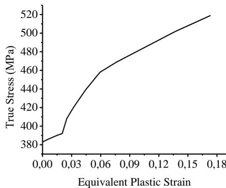
Fig. 3 – .Equivalent Plastic Strain and True Stress Relationships of Steel Tubes
