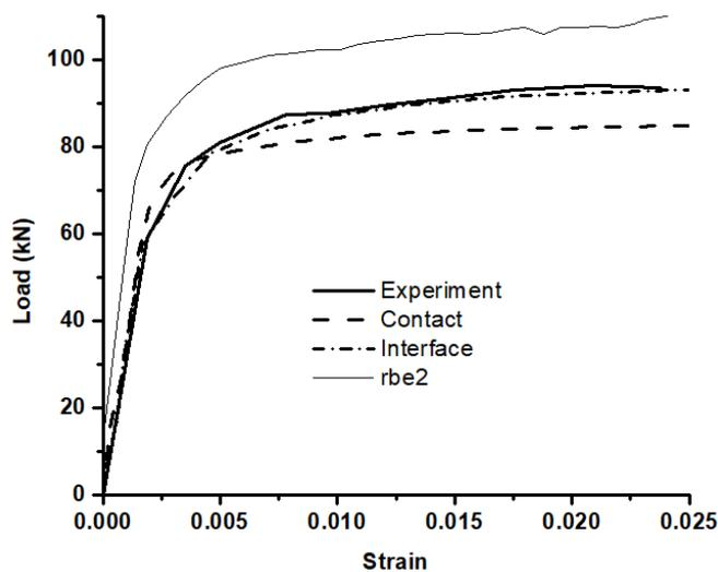
Fig. 12 – Load-Strain Relationships by Experiments and by Finite Element Analysis
