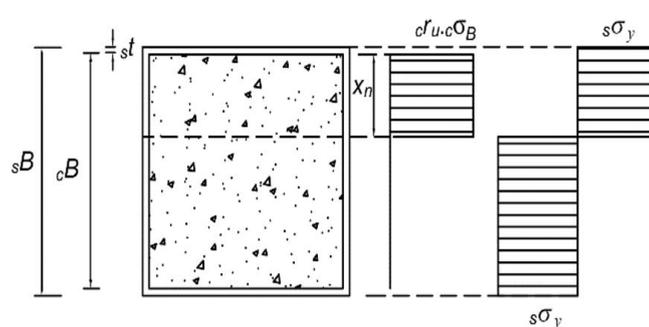
Fig. 9 – Stress Block for CFST Members' Ultimate Bending Capacity
