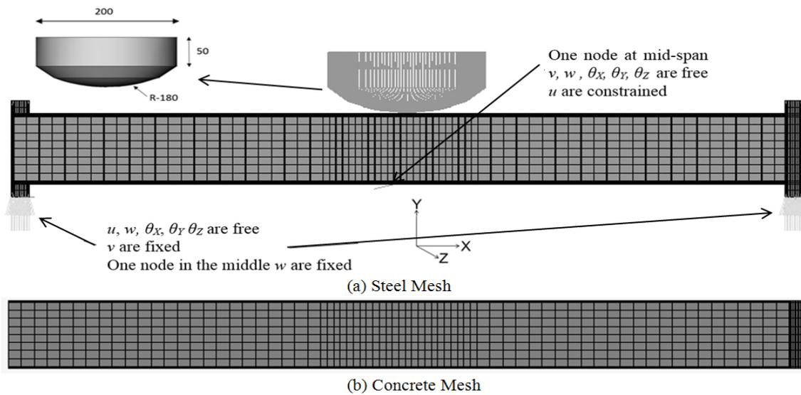
Fig. 5 – Boundary Conditions and Mesh Segmentation with Contact Analysis
