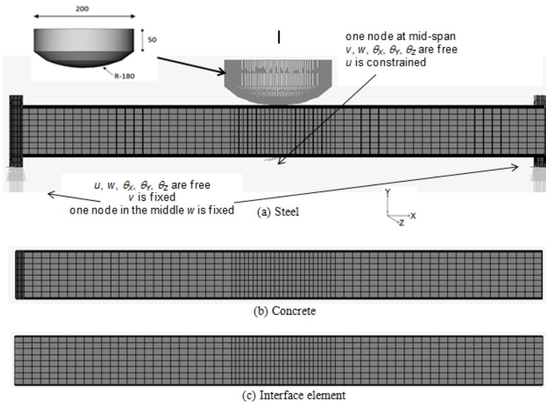
Fig. 6 – Boundary Conditions and Mesh Segmentation with Interface Element
