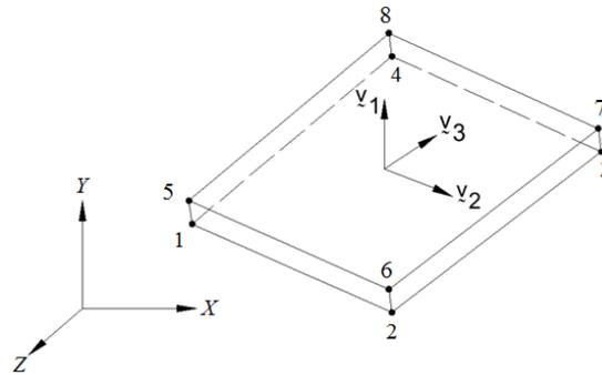
Fig. 8 – The connectivity of the interface element
