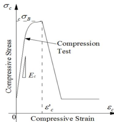
Fig. 4 – Concrete Model in Compressive Path
