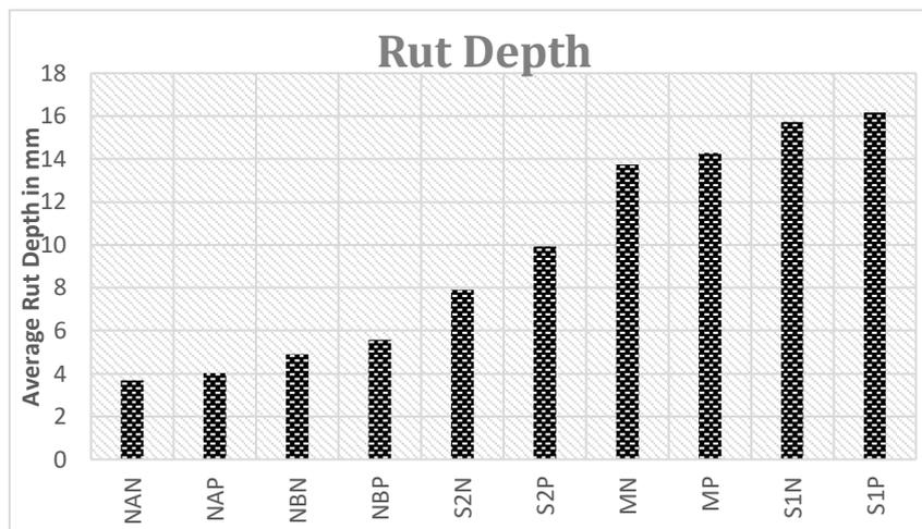
Fig. 4 – Average Rut Depth from Hamburg Wheel Tracker Test
