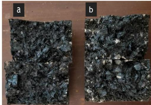
Fig. 3 – TSR Samples: (a) Unconditioned (b) After Conditioning
