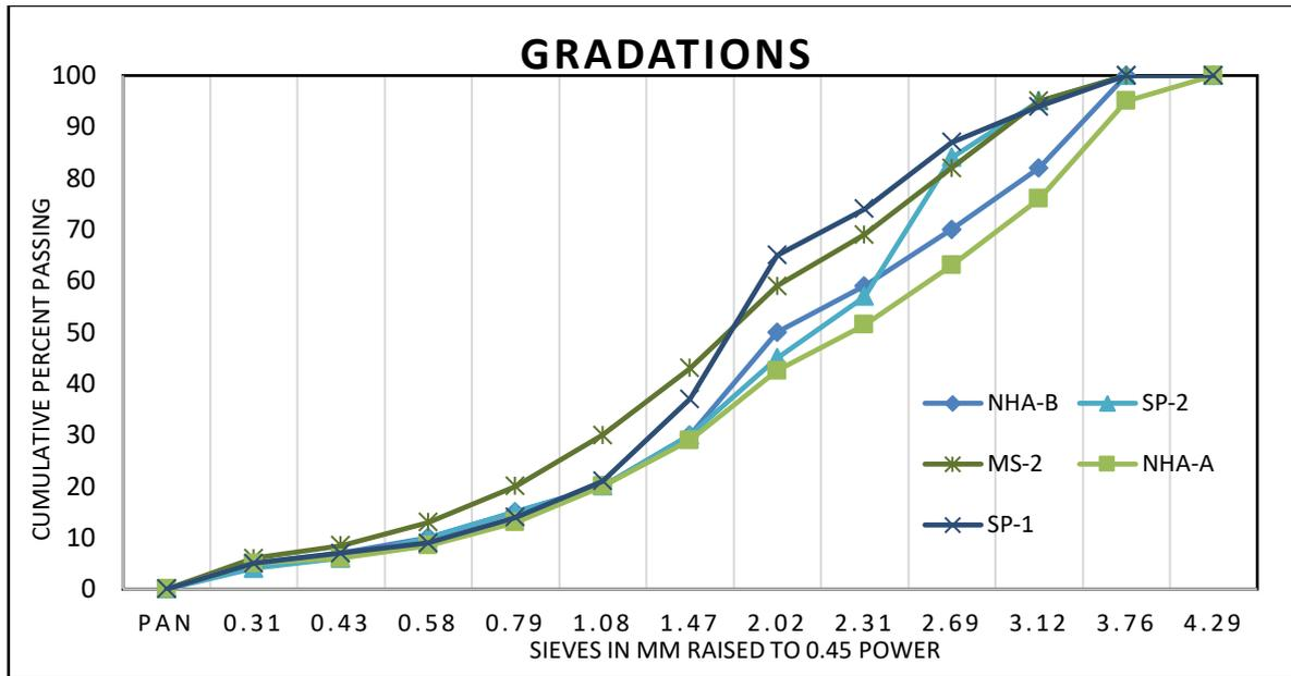
Fig. 1 – Aggregate gradations for asphalt wearing course
