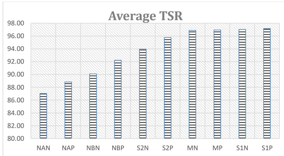
Fig. 6 – TSR values of different asphalt mixtures
