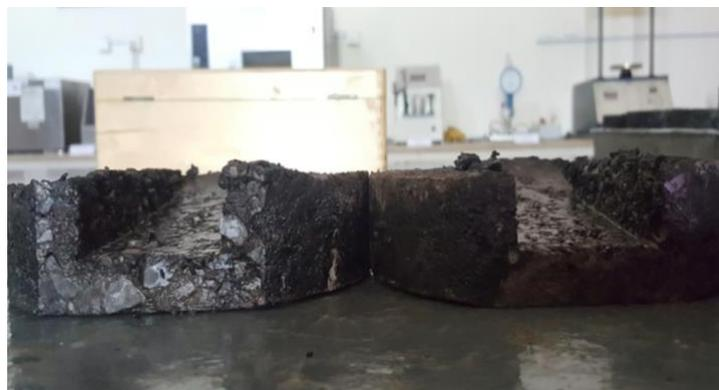
Fig. 2 – Hamburg Wheel Tracker Sample after Testing
