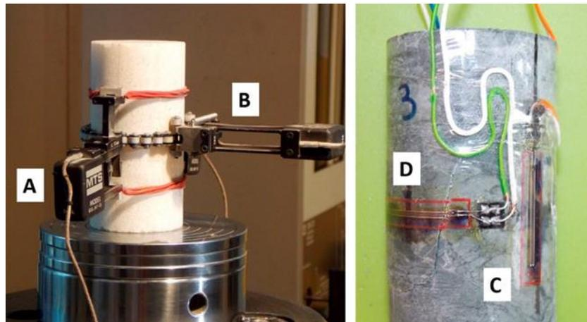
Fig. 1 – Examples of strain measurement sensors: Left – LVDTs; Right – strain gauges. A – axial LVDT; B – circumferential chain LVDT; C – axial strain gauge; D – radial strain gauge.
