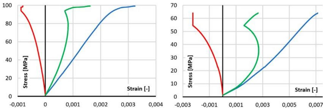
Fig. 3 – Stress-strain diagrams with components of the strains: Left – syenite; Right – sandstone; blue line – axial strain; red line – radial strain; green line – volumetric strain.
