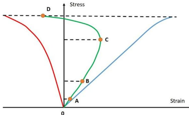
Fig. 2 – Behaviour of strain components: blue – axial strain; red – radial strain; green – volumetric strain (modified from [3], [4]).
