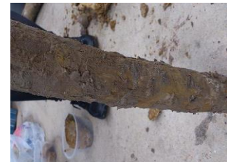
Fig.10 – Two test piles Fig.11 – Soil block from the glossy surface pile Fig.12 – Bonding layer
