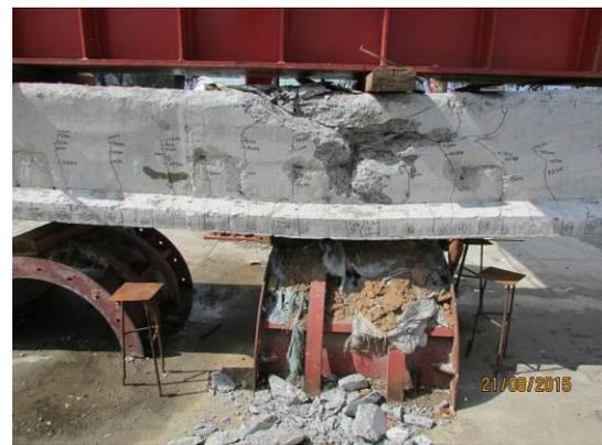
Fig. 3(b) - Failure state of beam M2-2
