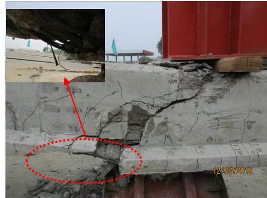
Fig. 4(b) - Failure state of beam M5.2-2
