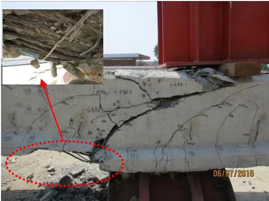
Fig. 4(a) - Failure state of beam M5.2-1
