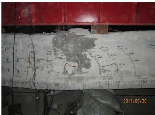
Fig. 3(a) - Failure state of beam M2-1
