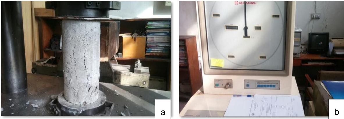
Fig. 3 – (a) & (b) Compressive test of concrete cylinder
