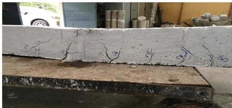
Fig. 8 – Crack pattern in 40% PCA specimen
