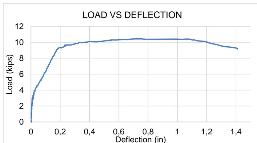
Fig. 5 – Average load vs. deflection curves for beams having W/C=0.68, PCA=0%
