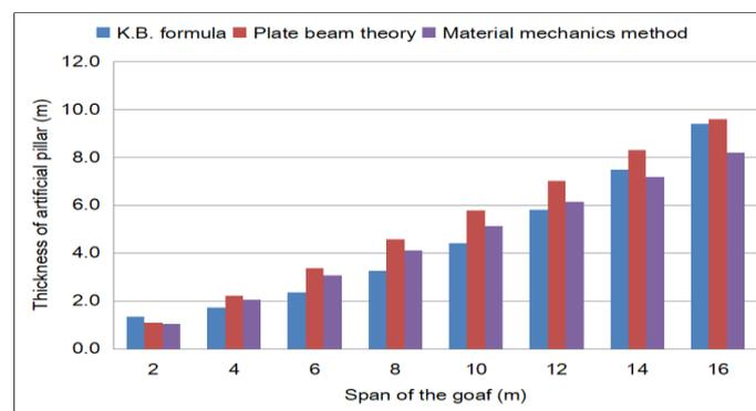
Fig.3 - Similar calculation results of artificial pillar thickness
