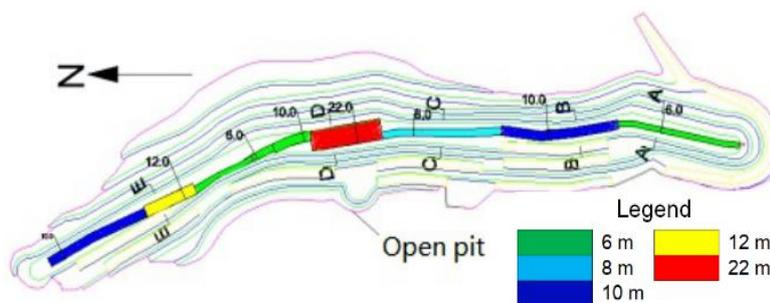
Fig.5 - Layout plan of artificial pillar
