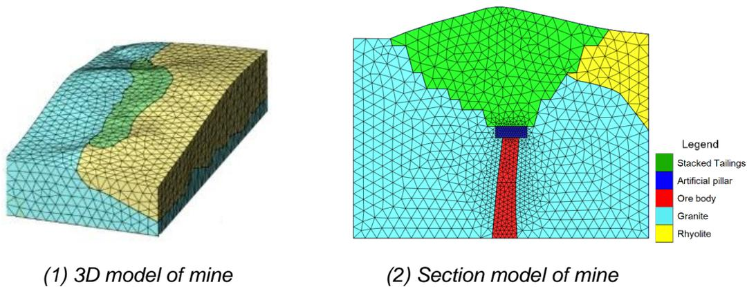
Fig.9 - The numerical simulation model based on MIDAS software
