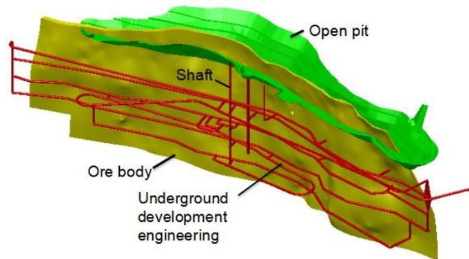
Fig.4 - 3D design model of transition from open pit to underground mining
