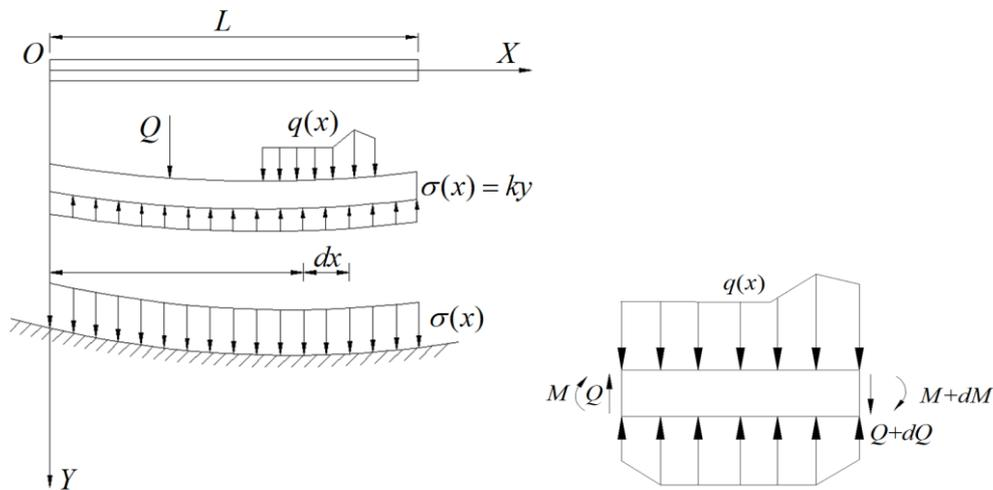
Fig.1- Microelement analysis of the boundary pillar model
