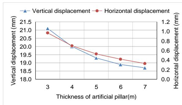
Fig.11 - The maximum displacement of artificial pillars at different thicknesses
