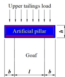
Fig.6 - Structure arrangement of artificial pillar      Fig.7 - Magnifying structure of artificial pillar
