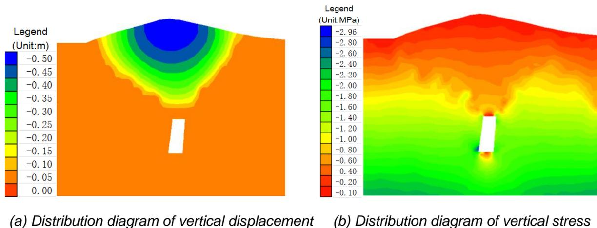
Fig.10 - The results of calculation by using FLAC3D software
