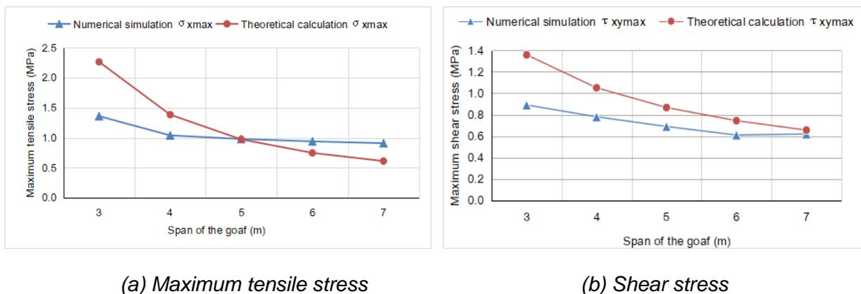
Fig.12 - Comparison between theoretical calculation and numerical simulation results
