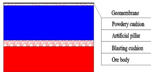
Fig.8 - The upper isolation layer and the lower cushion structure of artificial pillars
