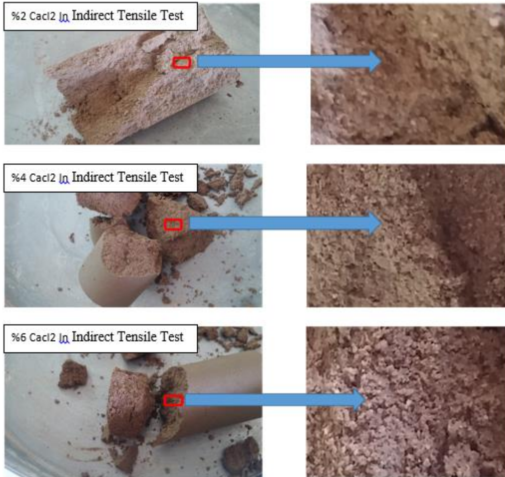
Fig.13 - Investigation of the free space amount at different percent of calcium chloride
