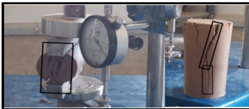
Fig.14 - The style of specimens fracture under indirect tension and unconfined compression test
