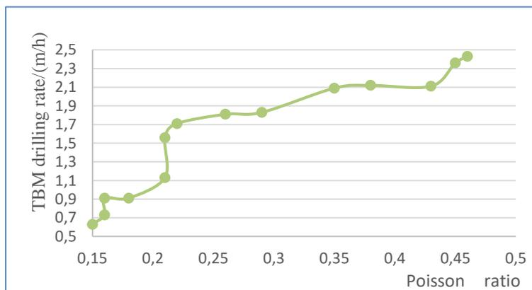
Fig. 4 - Relation diagram between the TBM driving rate and Poisson's ratio
