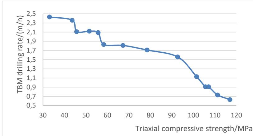
Fig. 2 - Relation diagram between the TBM driving rate and Triaxial compressive strength
