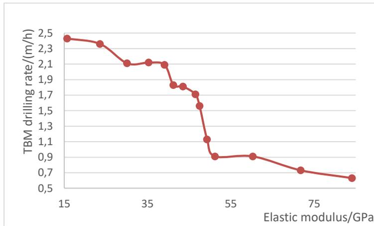
Fig. 3 - Relation diagram between the TBM driving rate and Elastic modulus
