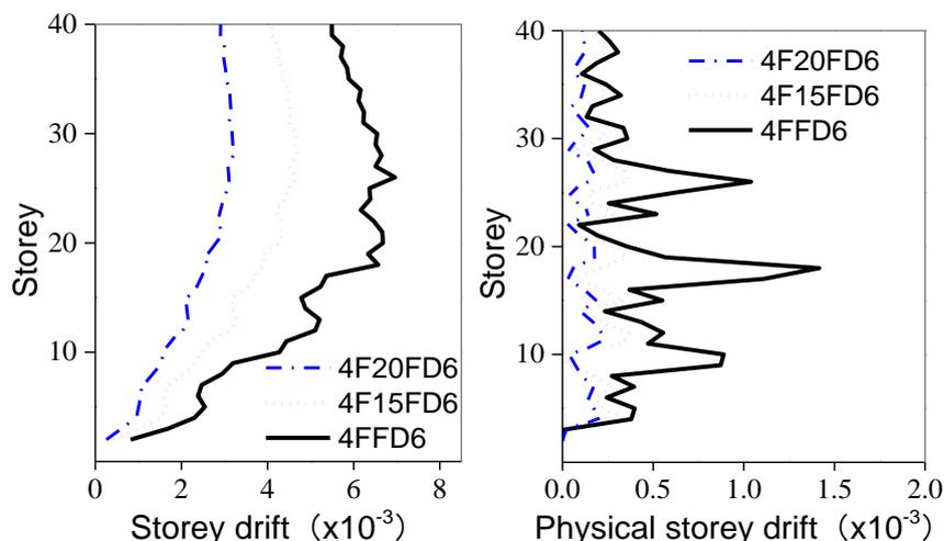
Fig.9 - Storey drift and physical storey drift under different diagonal column section (The diameters and wall thicknesses of the diagonal columns of the models 4FFD6, 4F15FD6 and 4F20FD6 are 1x, 1.5x and 2x, respectively, of the model 4FFD6)
