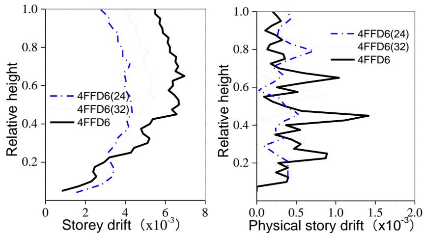
Fig.11 - Storey drift and physical storey drift under different structure aspect ratio (The structural aspect ratios of the model, 4FFD6(24), 4FFD6(32) and 4FFD6 are 2.67, 3.56 span and 4.44, respectively)
