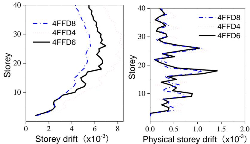
Fig.10 - Storey drift and physical storey drift under different main ring beam span (The structural main ring beam spans of the models 4FFD4, 4FFD6 and 4FFD8 are 4 spans, 6 spans and 8 spans)
