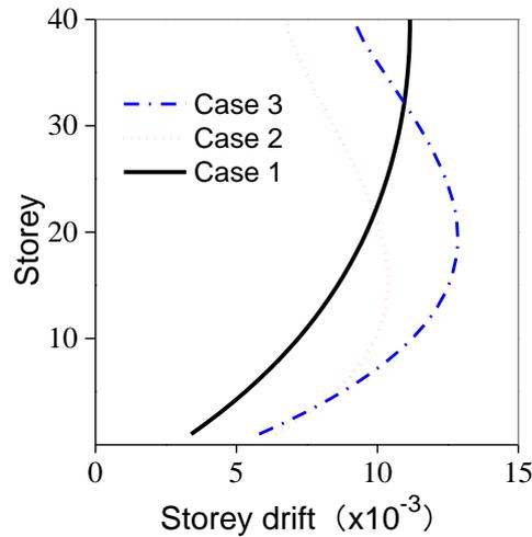
Fig.5 - The storey drift under 3 cases
