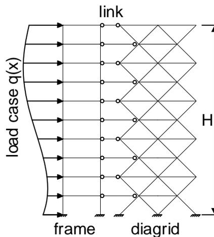
Fig.1 - Simplified analysis model for the frame-diagrid structure
