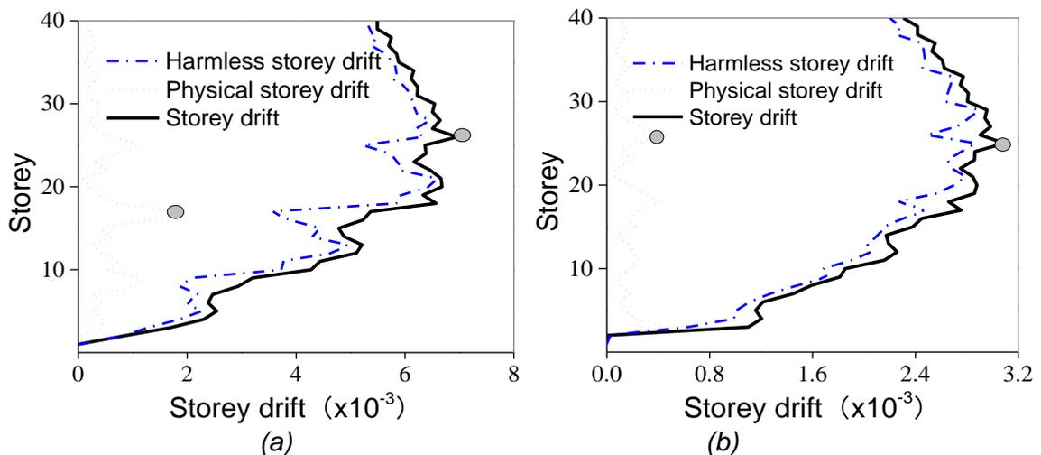
Fig. 6 - Storey drift of model 4FFD6 (a) during frequently earthquakes (b) during rarely earthquakes
