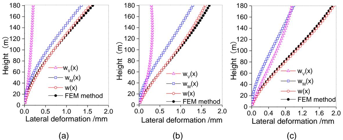
Fig. 4 - Result of lateral deformation. (a) Case 1: Top point lateral load (b) Case 2: Uniform distributed lateral load and (c) Case 3: Reverse triangle distributed lateral load
