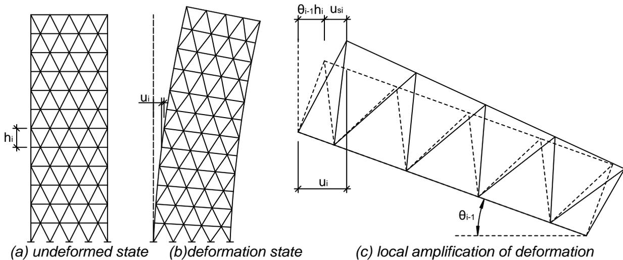
Fig.2 - High-rise frame-diagrid structure lateral deformation
