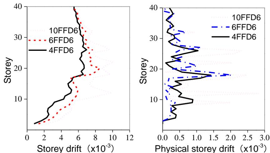
Fig.8 - Storey drift and physical storey drift under different diagonal column angles (The angles of the diagonal columns of 4FFD6, 6FFD6 and 10FFD6 is 68°, 75° and 81°, respectively)
