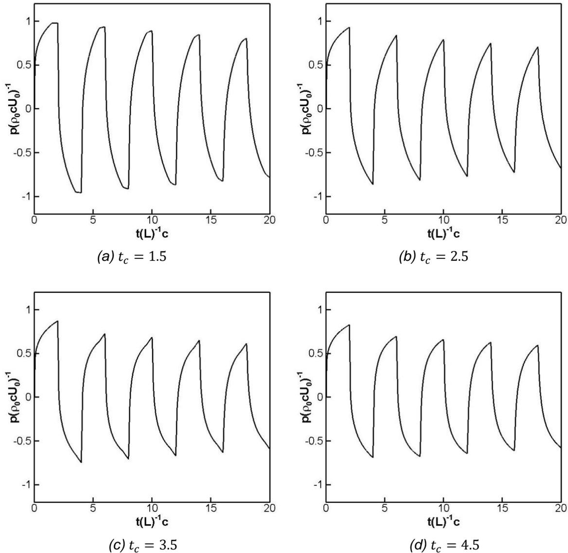
Fig. 6 - Pressure  $p$  at valve end with  $m = 0.2$  and different closing time.
