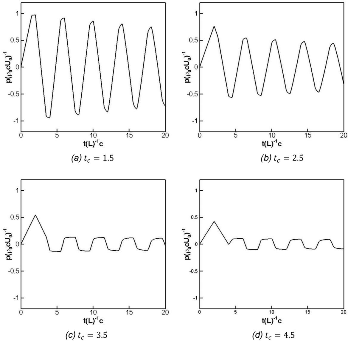
Fig. 7 - Pressure  $p$  at valve end with  $m = 1$  and different closing time.
