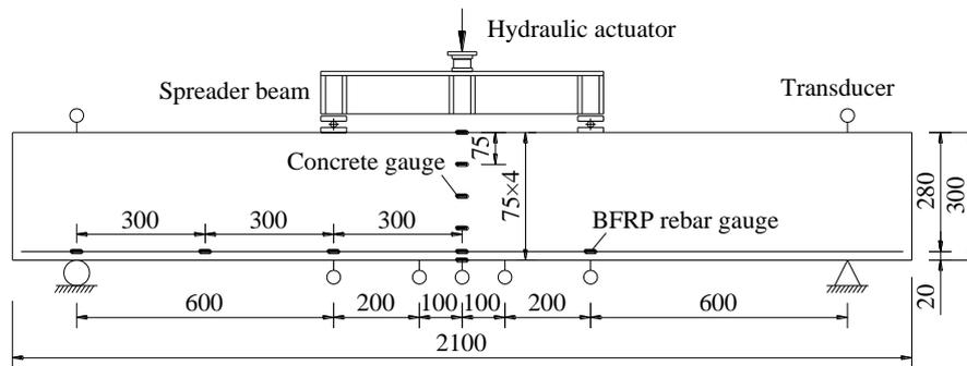
Fig. 2 - Details of test beam and setup
