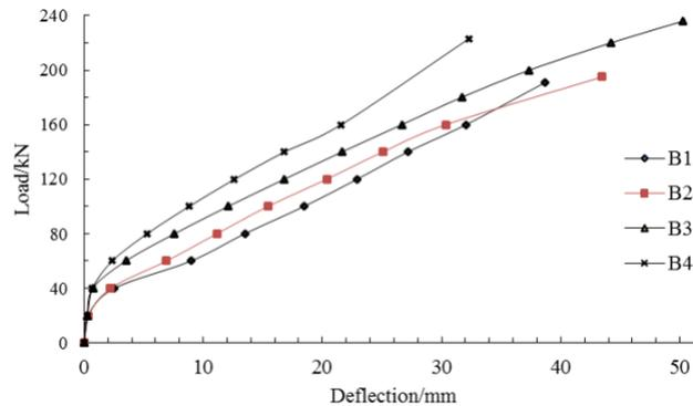
Fig. 4 - Load-deflection relationship for different dosages of steel fibre
