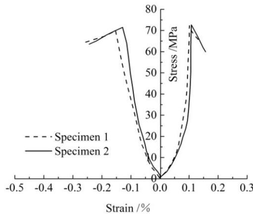
(c) The stratification plane is parallel to the axial direction of the specimen
