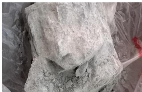
Fig. 2 - Weathered argillaceous slate
