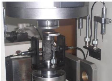
*Fig. 1 - RMT-150 Compression Machine*
