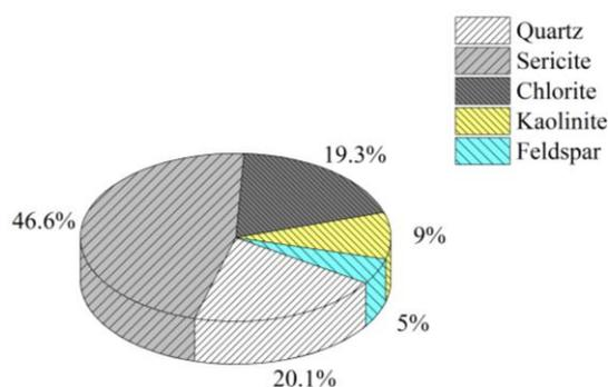
Fig.3 - Mineral composition of argillaceous slate
