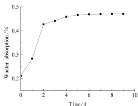
Fig.4 - The relationship between water absorption and time
