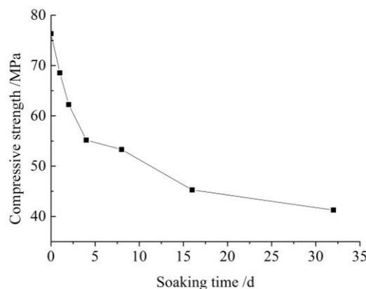
*Fig. 7 - Relationship curves between strength and saturated time*
