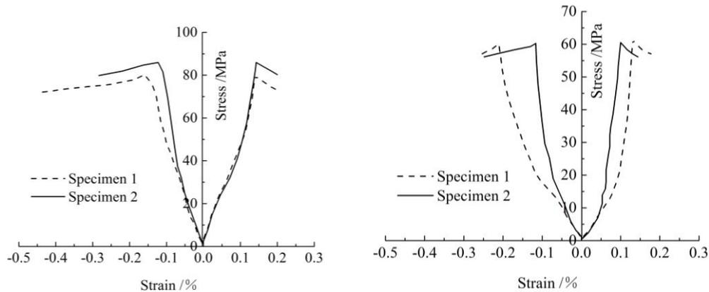
(a) The stratification plane is perpendicular to the axial direction of the specimen
