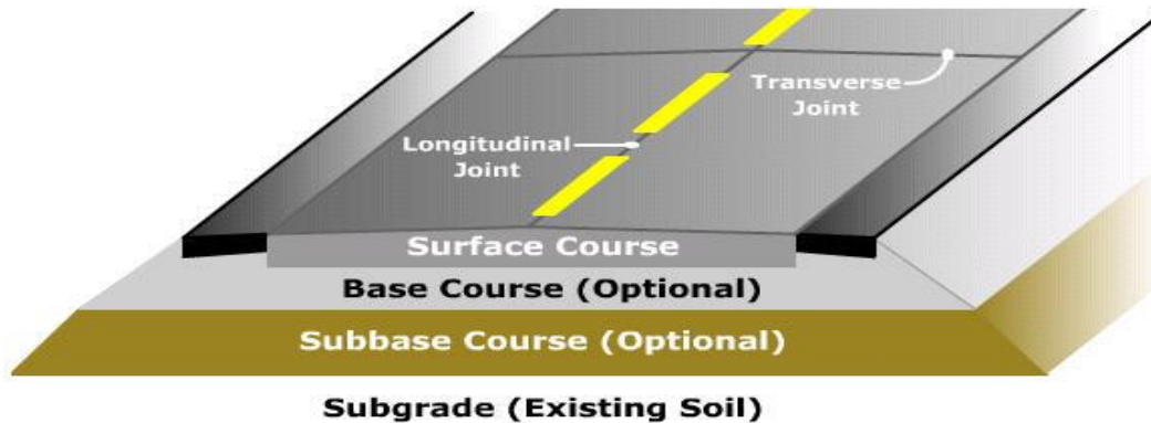
Fig. 1 - Typical Concrete Pavement Sections [13].
