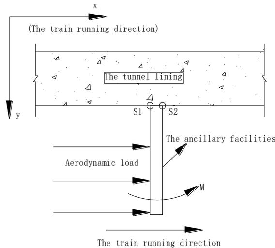
Fig. 4 - Force analysis and measuring point position of bolt anchored catenary under aerodynamic load
