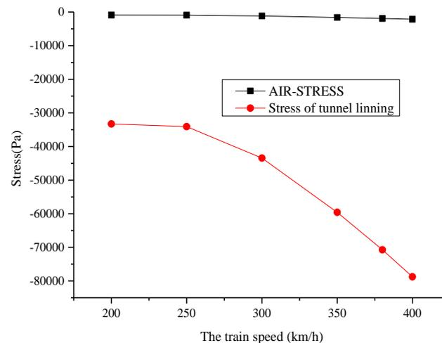
Fig. 8 - Maximum negative pressures in X direction of tunnel lining structure
