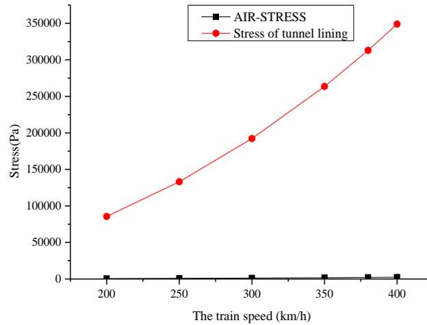
Fig. 9 - Maximum positive pressure in Y direction of tunnel lining structure
