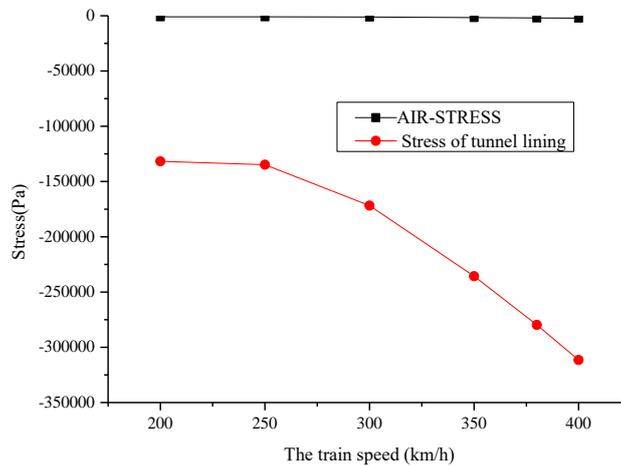
Fig. 10 - Maximum negative pressure in Y direction of tunnel lining structure
