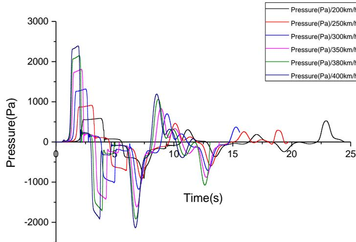
Fig. 2 - Calculation results of aerodynamic loads at different speeds
