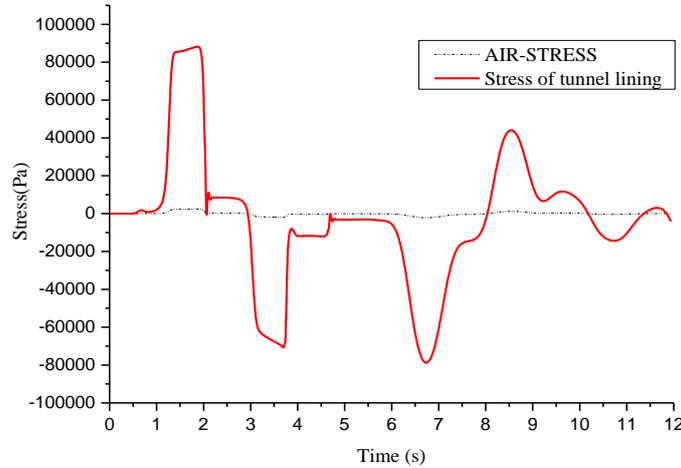
Fig. 5 - The stress of X direction when the train speed is 400km/h
