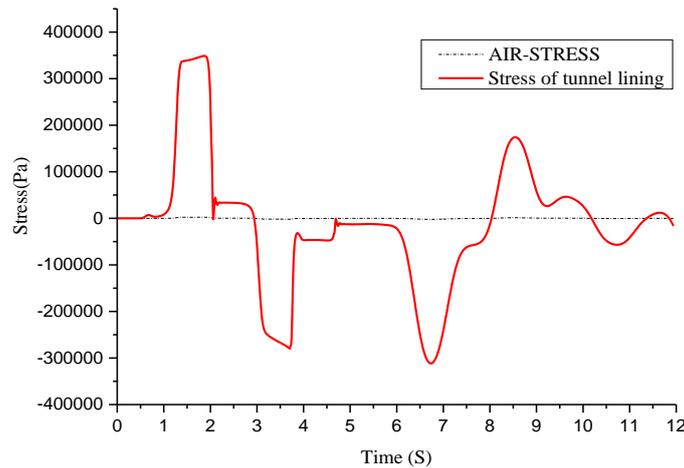
Fig. 6 - The stress of Y direction when the train speed is 400km/h
