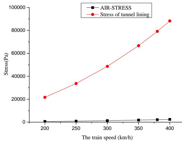
Fig. 7 - Maximum positive pressure in X direction of tunnel lining structure
