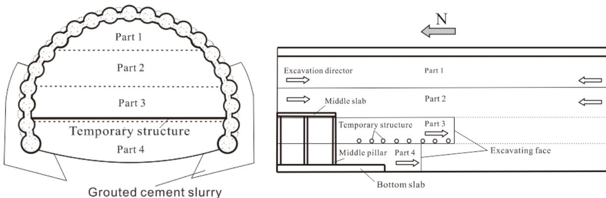
Fig.8 - Large cross-section excavation
