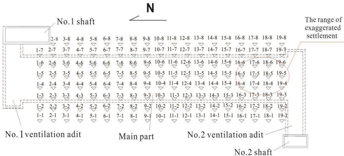
Fig.2 - Plan of Xinleyizhi Station and sections layout of settlement monitoring
