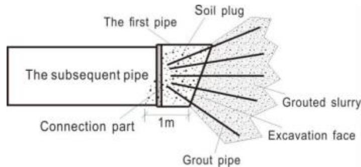
Fig.9 - Pre-grouting at the loose and saturated section
