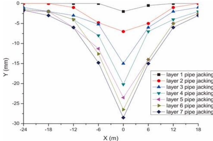
Fig.5 - Typical accumulated transverse surface settlement curve in STEP1
