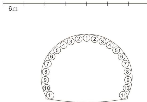
Fig.3 - Monitoring points layout of each section
