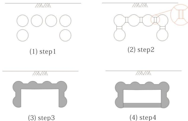
Fig.1 - Construction process of PPM
