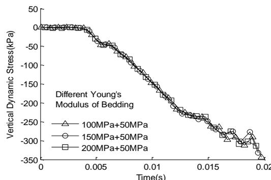
Fig. 4 - The effect on dynamic stress of pile top subgrade of elastic modulus
