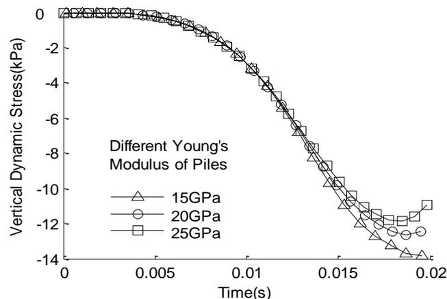
Fig. 11 - Effect of dynamic stress on soil between piles of pile elastic modulus
