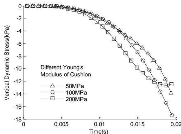
Fig. 7 - Effect of cushion elastic modulus on dynamic stress of soil between piles
