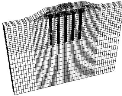
Fig.2 - Three-dimensional finite difference model of pile-soil composite foundation
