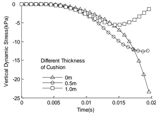
Fig. 9 - Effect of cushion thickness on dynamic stress of soil between piles
