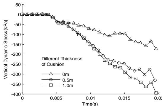
Fig. 8 - Effect of cushion thickness on dynamic stress of pile top
