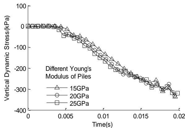
Fig. 10 - Effect of dynamic stress on pile top of pile elastic modulus
