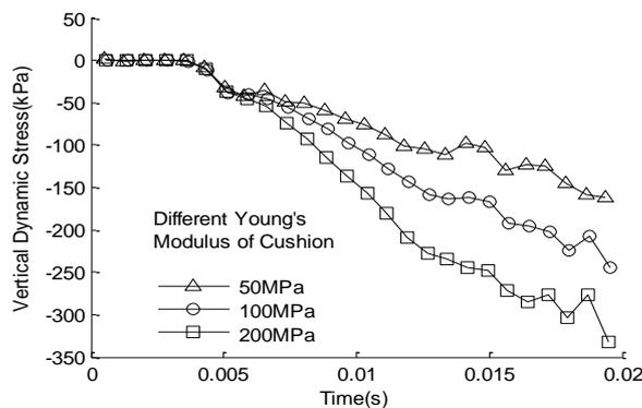
Fig. 6 - Effect of cushion elastic modulus on dynamic stress of pile top
