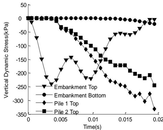
Fig. 3 - Dynamic stress time history curves of pile and embankment
