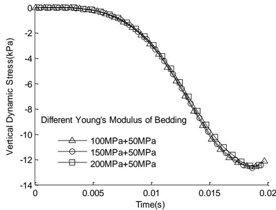
Fig. 5 - Effect on dynamic stress of soil between piles of subgrade elastic modulus
