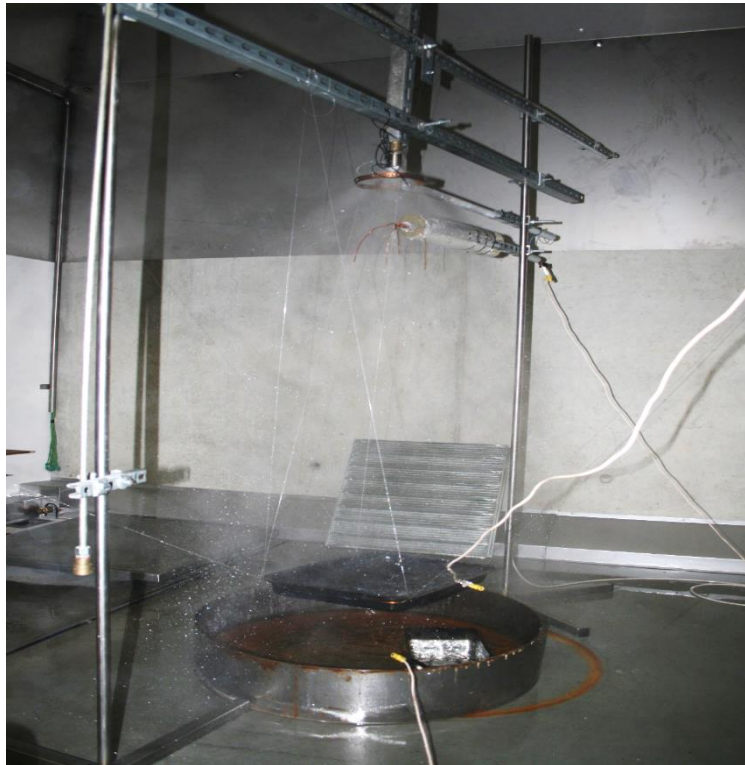
Fig. 1 - A look at the test equipment at the time of extinguishing the burning of n-heptane in a metal tray
