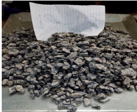
Fig. 3 - Sample of coarse aggregate used.
