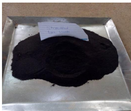
Fig. 5 - Sample of ground tire used.
