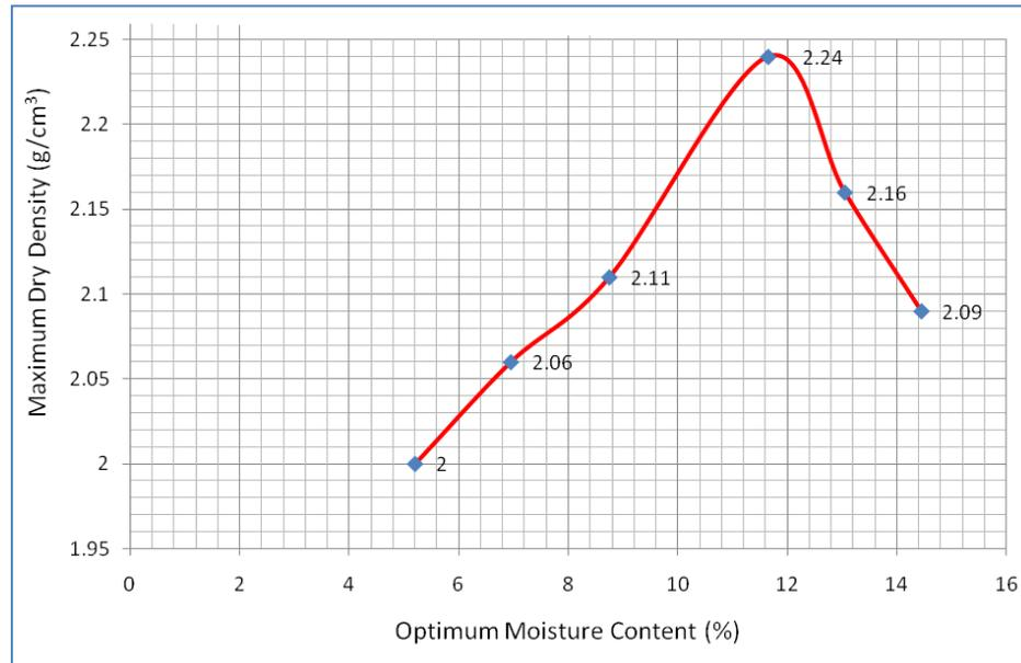
Fig. 3 - Compaction curve for the natural lateritic soil
