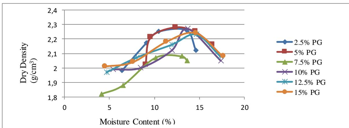
Fig. 5. - Compaction curves for the soil with varying PG content
