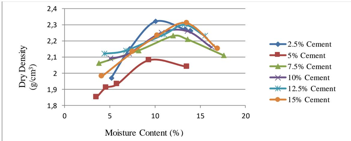
Fig. 6. - Compaction curves for the soil with varying cement content
