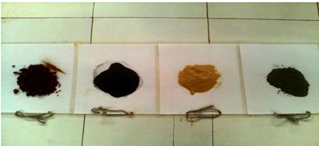
Fig. 1. - Samples of laterite, rice husk ash, powdered glass and cement
