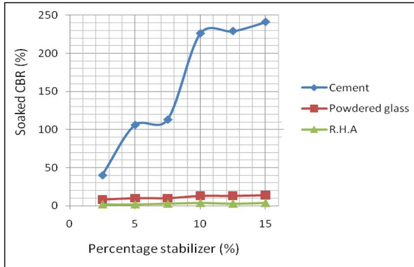
Fig. 8. - Soaked CBR curves for the soil with varying additives
