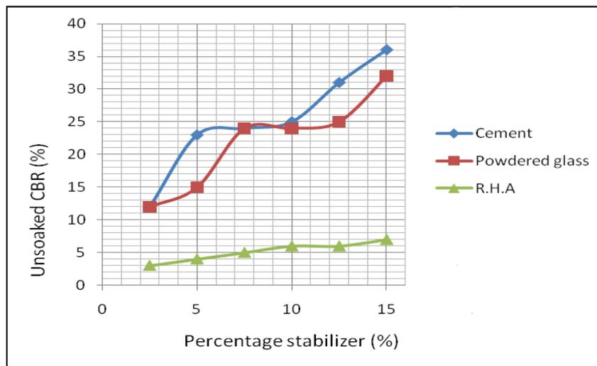
Fig. 7. - Unsoaked CBR curves for the soil with varying additives
