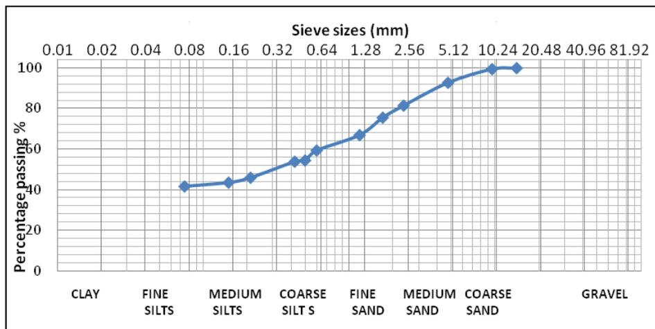
Fig. 2. - Particle Size Distribution chart for the lateritic soil
