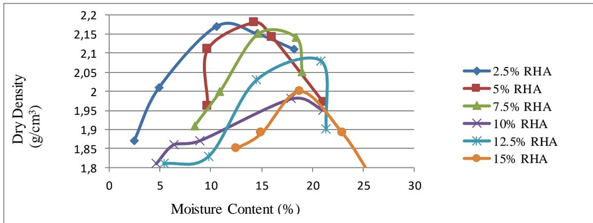
Fig. 4. - Compaction curves for the soil with varying RHA content
