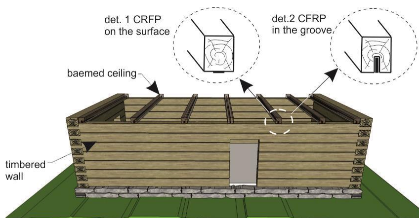
Fig. 5: Securing the spatial rigidity of a timbered construction in the case of degraded tie beams – reinforcing FRP strips or lamellae are led along the surface or in the groove of joists and anchored to the outside
